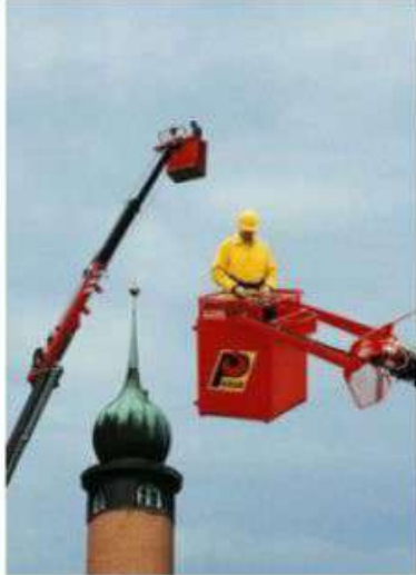
Work platform assembled with a variable reach lift truck
